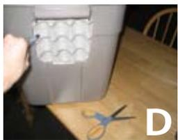
**Cut egg carton from doorway (Step D):** Trace the plastic opening with a felt pen and then using scissors cut through the egg carton to match the dimension of the bin opening.
